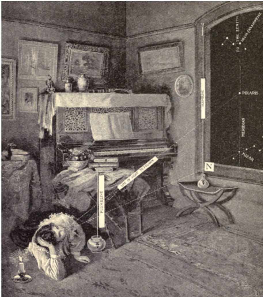
Finding True North without Clock or Telescope (from a Photograph by Lovell)
